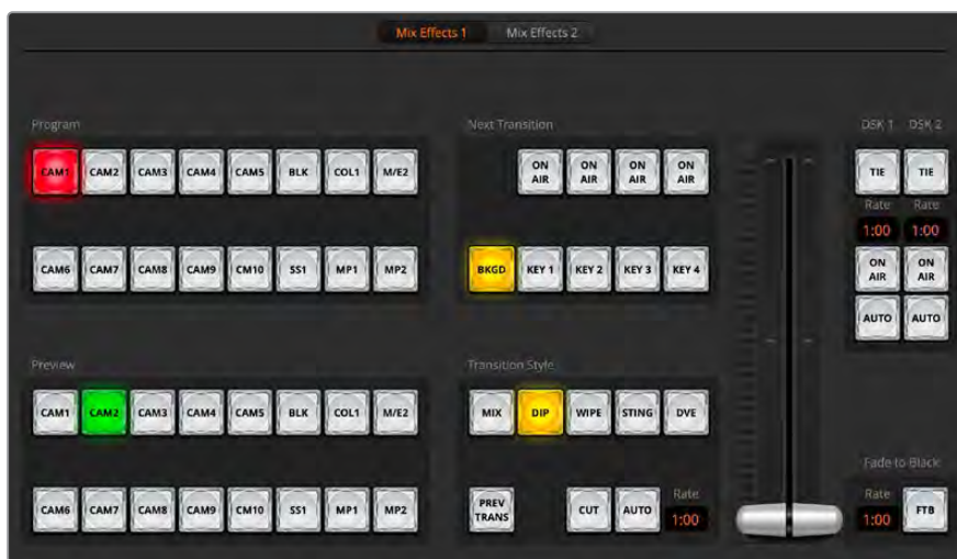
On ATEM 2 M/E and 4 M/E models, select the mix effects panel using the numbered buttons at the top of the interface
